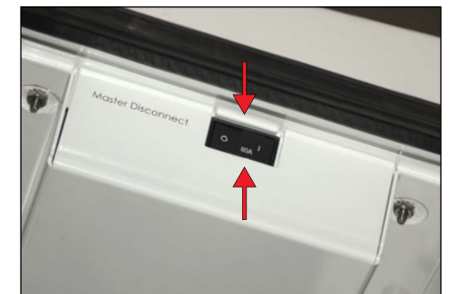
FIGURE 3 Main power ON/OFF switch.
